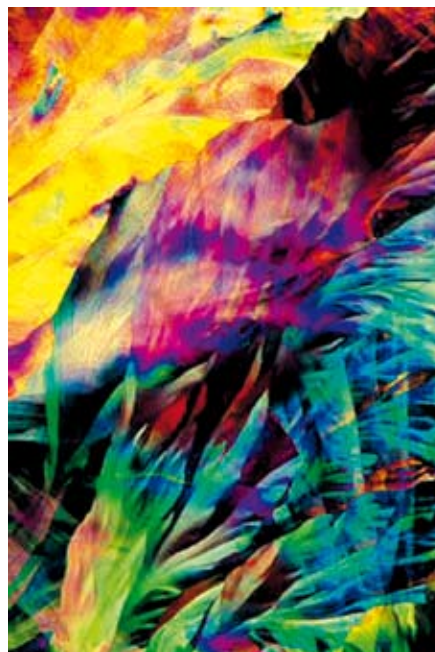
Fig. 37: Transmitted polarising microscopy; variation of melted chemicals viewed with crossed polariser. Images courtesy of Norbert Junker, Olympus Europa GmbH, Hamburg, Germany.
